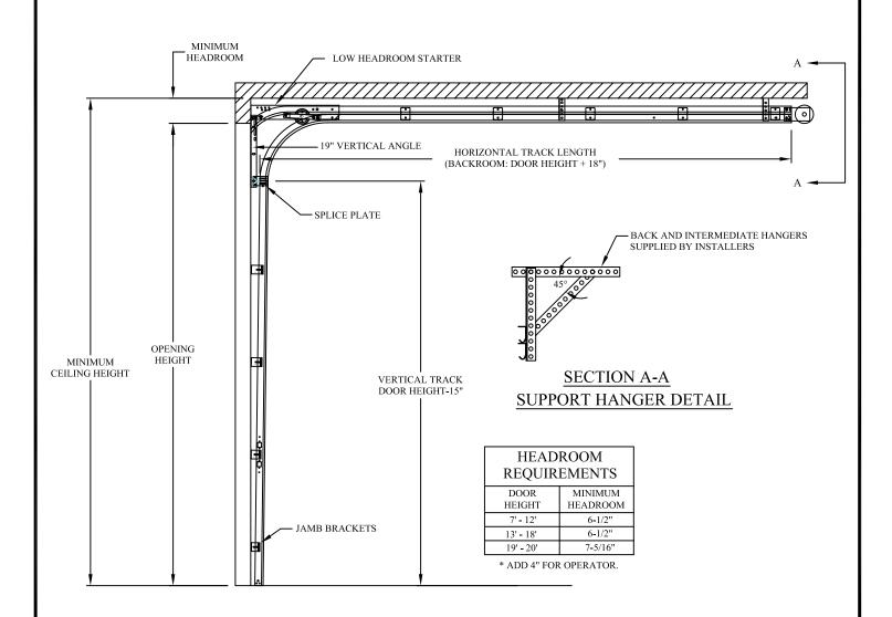
STANDARD LIFT LOW HEADROOM TO THE REAR BRACKET MOUNT TRACK SET DETAIL
