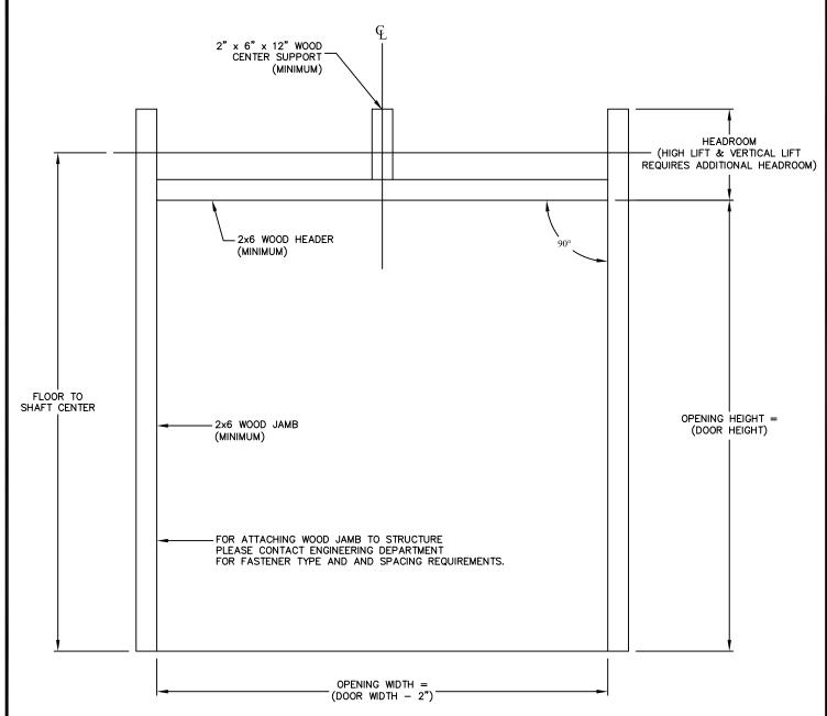
1) FOR DOORS REQUIRING MORE THAN TWO SPRINGS, ADDITIONAL SPRING PADS MAY BE NEEDED.
