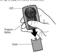
4 Press and release the button. When the LED stops flashing, continue to press and release the button until a click is heard from the garage door opener, a light on the garage door opener blinks, the garage door opens/closes, or a beep is heard from the gate operator (maximum 18 times).
