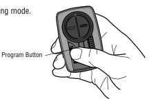
Open the remote control by sliding the battery cover down. Press and hold the program button until the LED lights (approximately 2 seconds).
